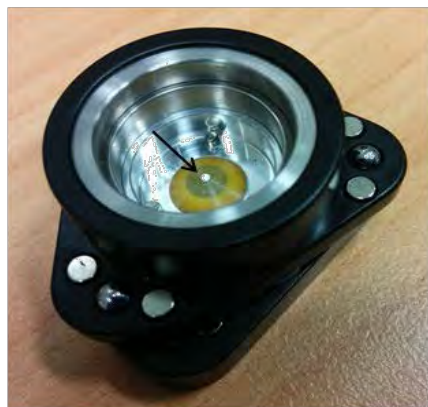
Underside of ATR crystal showing 1mm contact facet (arrow)
