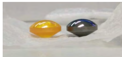
Custom ZnSe and germanium ATR crystals
