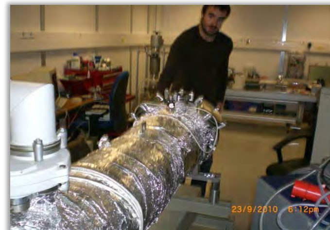
Multipass room temp cell at Soleil Optical Path Length ~ 152 m
