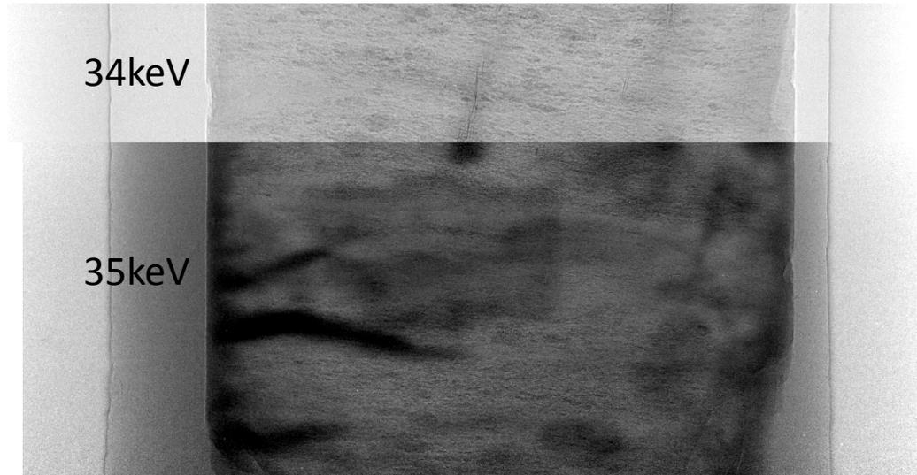
By subtracting the image taken below the absorption edge from that above, the contribution to the image from the contrast agent (or element of interest) is isolated. The x-ray attenuation of other materials does not change significantly between above and below the absorption edge
