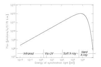
An electron energy of 3 GeV was chosen for the Australian Synchrotron storage ring to allow for the production of light at frequencies that encompass a wide range of the electromagnetic spectrum, from far infra-red to hard x-rays.
