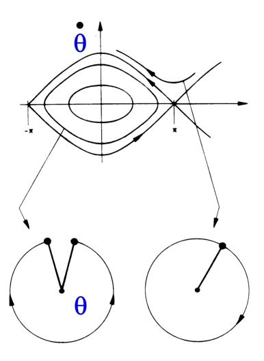
The "bucket" of synchrotron motion is just that of the rigid pendulum
