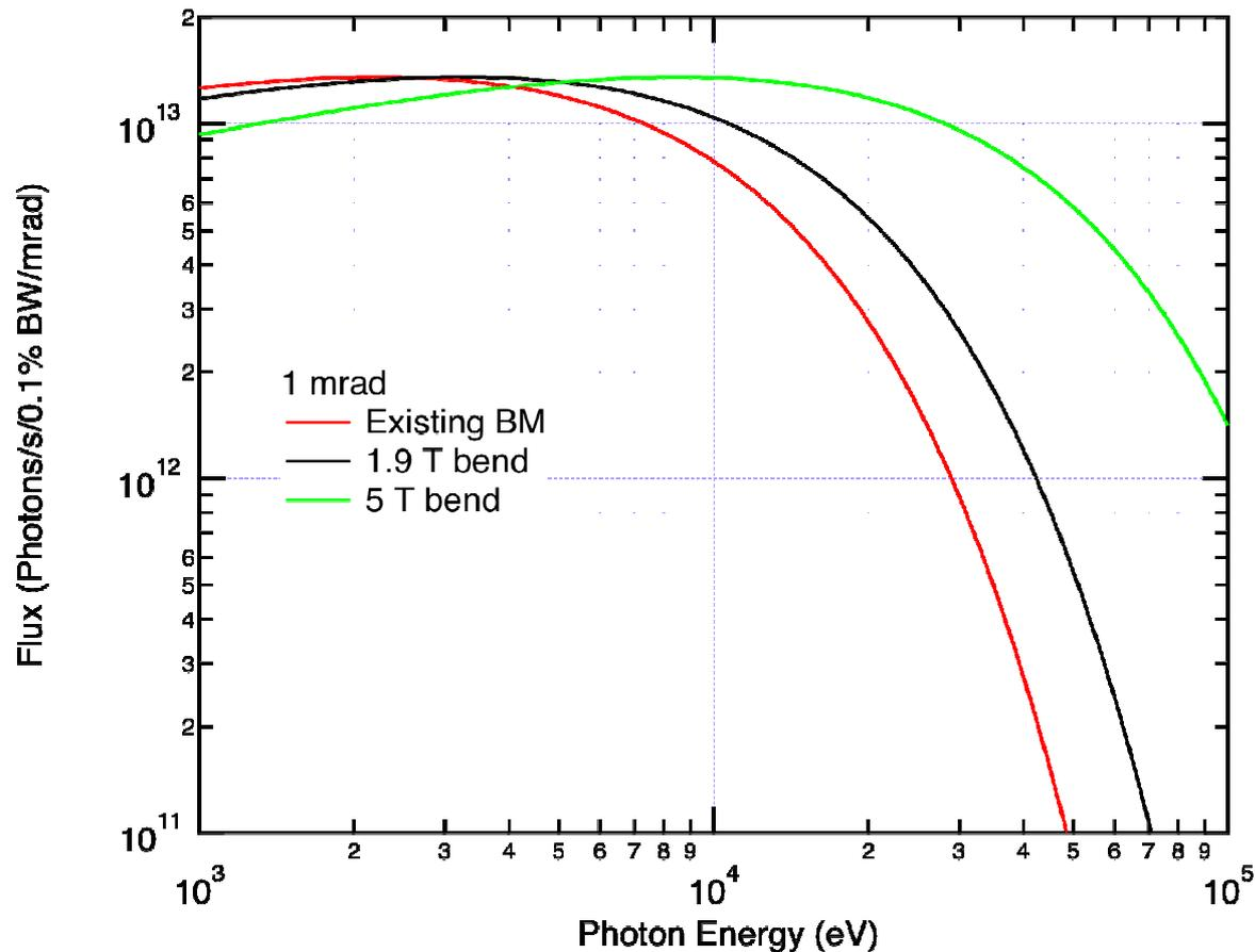
**Fig 1** A comparison of the estimated flux from an existing bend magnet at the Australian Synchrotron, a 1.9 Tesla bend magnet and a 5 Tesla superbend. The stored current is 0.2 A.
