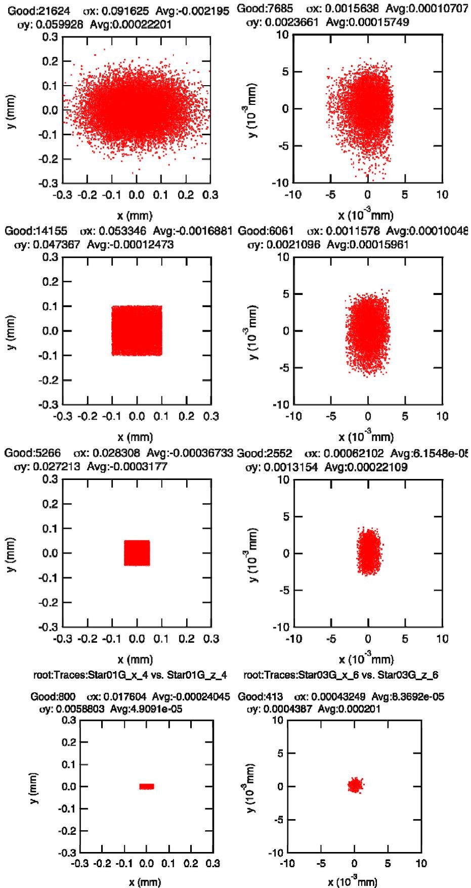
**Fig. 4** The pairs of figures show the spot size at the intermediate slit and its image after the KB pair. In the captions above the figures are RMS values.
