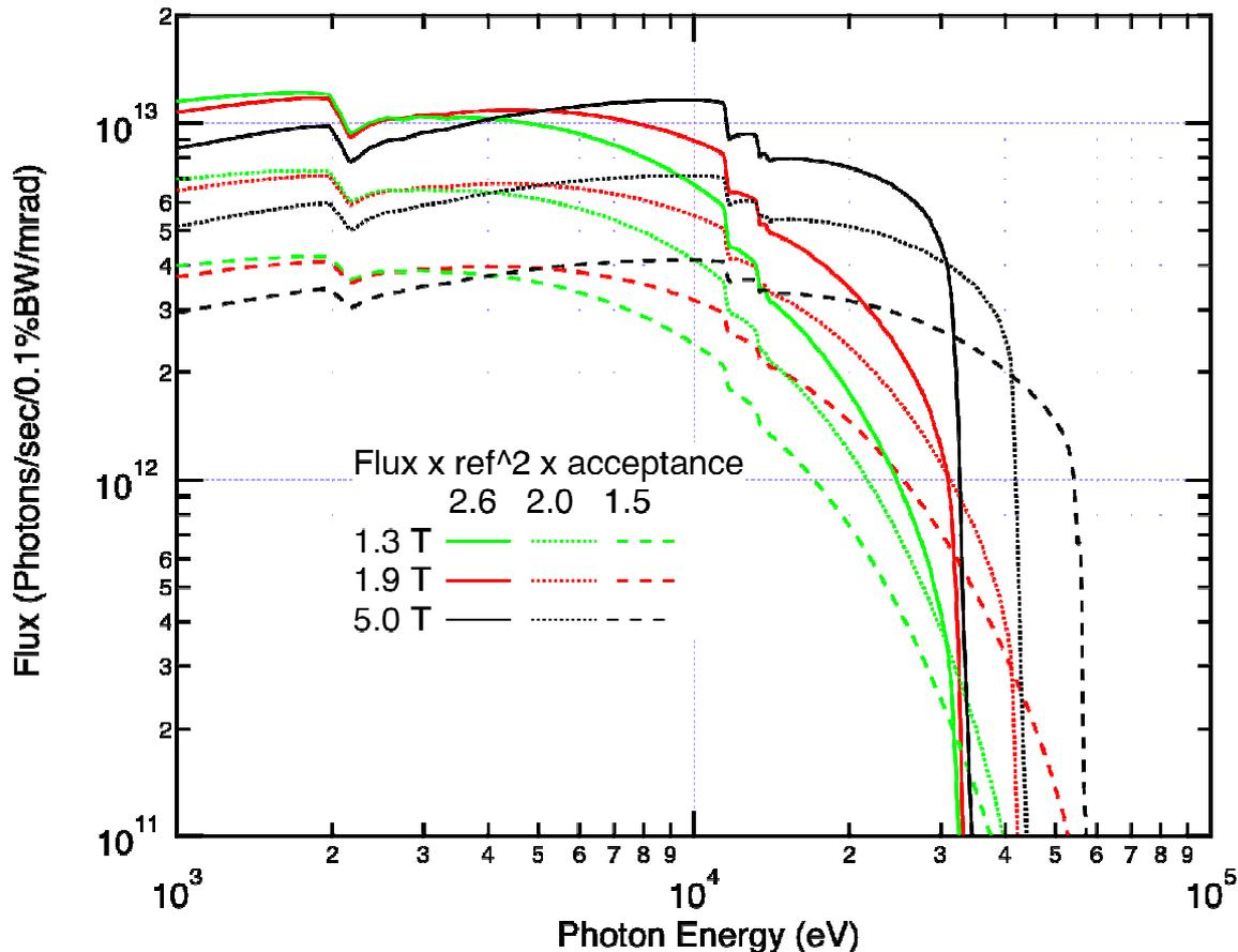
Fig. 3 Convolution of X-ray source and optics incident X-ray angle for 3 consecutive Pt coated optics devices (1 mrad acceptance, same length mirrors).
