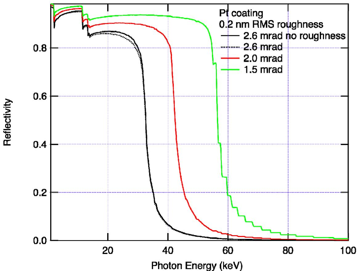
Fig. 2 Reflectivity of Pt coated mirrors at various angles of X-ray incidence.
