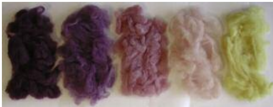
Merino wool dyed with different sizes of “nanosilver”. Photo: Victoria University of Wellington
