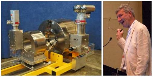
Above Left: 9 Tesla and 0.8 Tesla magnets for the LARIAT NEXAFS system at NSLSII Brookhaven National Lab. Designed and constructed by HTS-110 Ltd, New Zealand. Above Right: Jeff Tallon, IRL
