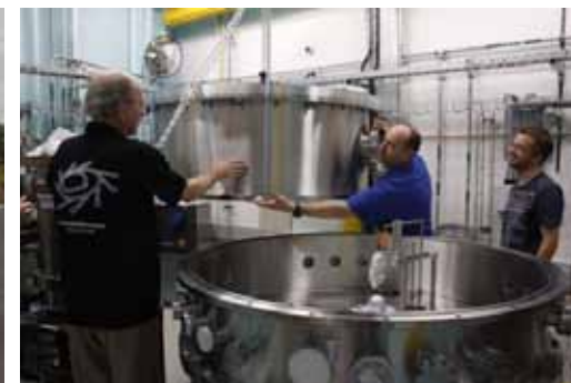
Above (L-R): John Bockwinkel (ANU), Jason Wirthensohn (AS) and Jonathan McKinlay (AS) prepare to place the upper half of the monochromator on the lower half transport tunnel
