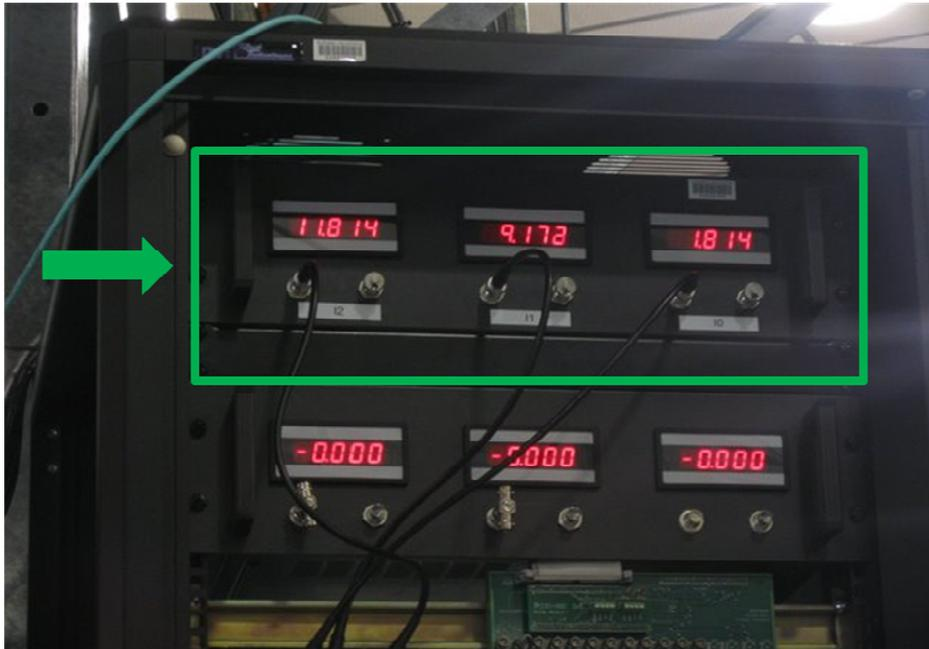
You should adjust the keithley (Keithley1, Keithley2 and Keithley3 for I0,I1 and I2, respectively) gains in order for these values to be in the right range. Click on the keithley button in the endstation GUI
