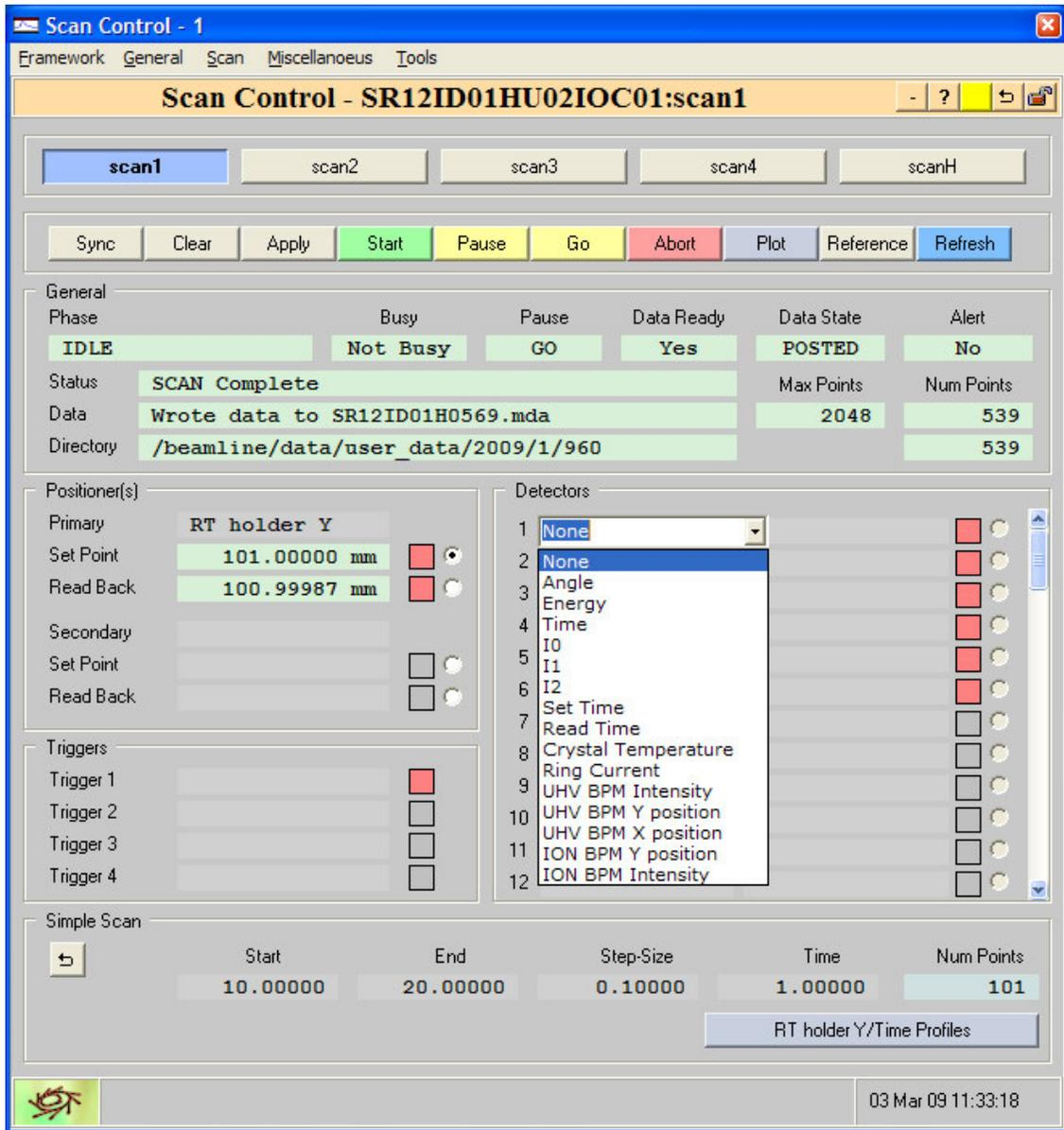
For scanning the positions you need I0, I1, I2, which are related to the incoming beam, the flux after the sample, and the flux after the reference, respectively.
