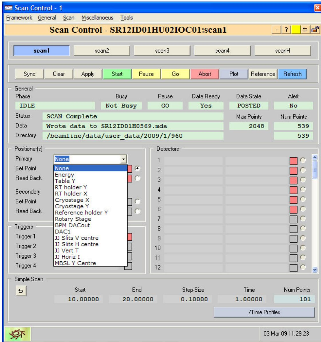
Select: RT holder (x and y) if you are performing measurements at room temperature; Cryostage (x and y) if you are measuring at cryotemperature.
