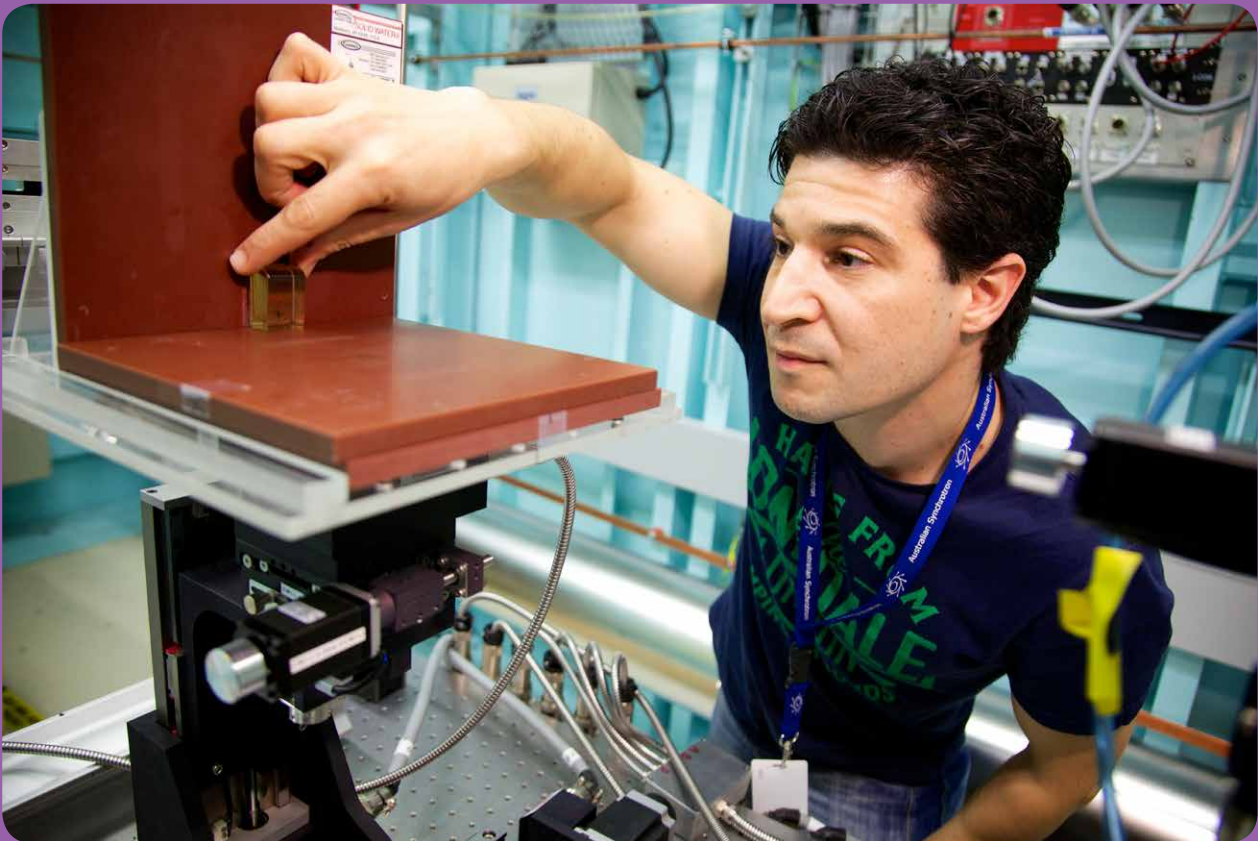
Frank Gagliardi is a Medical Physicist from the William Buckland Radiotherapy Centre at the Alfred Hospital and cancer researcher at RMIT University. Here on the Australian Synchrotron's Imaging and Medical Beamline (IMBL), he places a sample of radiosensitive human-tissue-equivalent plastic on the sample table. Frank is working with the IMBL team to understand the 3D dose distribution of x-ray microbeams, which will help develop new ways of treating cancer using synchrotron radiation.
