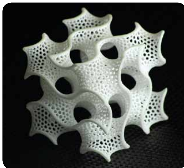
Pictured above is a 3D printed model of an advanced nano-structured material which assembles and encapsulates bioactive molecules (Conn and Drummond)
